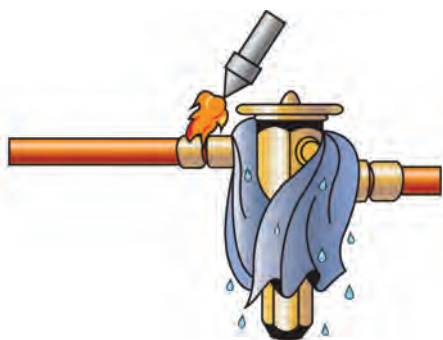
Figure 5 Wrap the valve with wet rags to avoid overheating.
